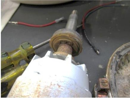
Figure 2: Rust on inboard bearing face that could be prevented by Triple Seal™ Protection
