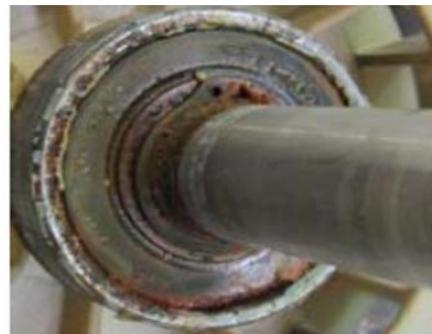
*Figure 1: Rust on bearing face is a sign of water intrusion*
