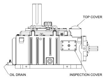
Figure 1 — Oil Drain and Cover Locations
