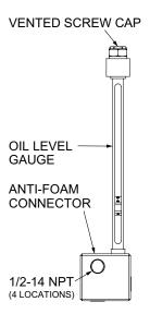
Figure 2 — Oil Level Gauge Assembly
