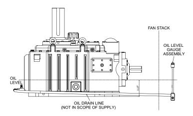
Figure 3 — Oil Level Gauge and Drain Line
