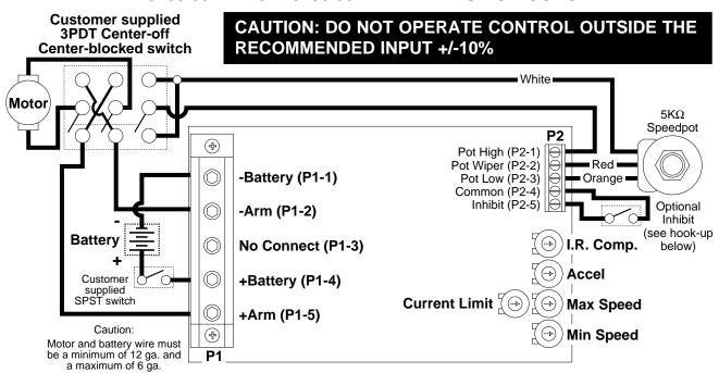
Relays may be used in place of switch, but a neutral position must be provided to prevent plug reversing. DO NOT ENGAGE OPPOSITE DIRECTION UNTIL MOTOR HAS COME TO A COMPLETE STOP. Failure to do so may result in damage to the control.
