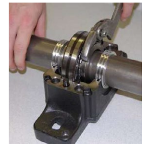
Figure 2 — Tighten Until Snug
