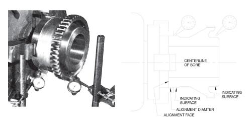
The alignment diameter of the hub should be chucked in the boring lathe and dial
