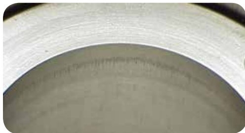
Image 5 – Repairable bore damage
