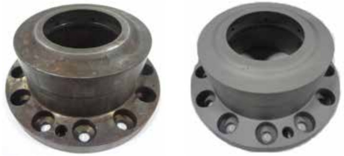
Image 6 – Coupling hub before and after bead blasting
