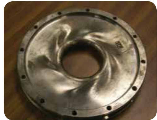
Image 4 – Rippling on diaphragm profile due to torque overload.
