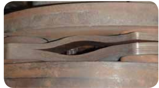
Image 3 – Unacceptable spreading in disc pack
