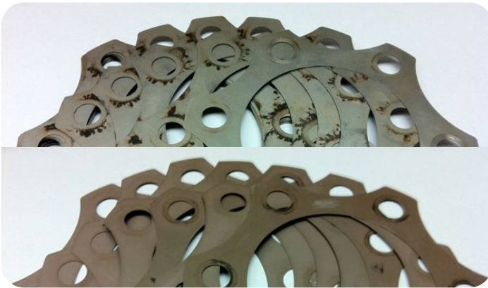
Image 5 – No coating on top, low friction coating on bottom
